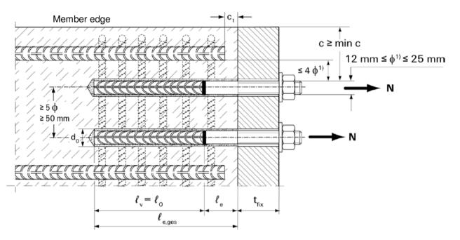
$^{1)}$  If the clear distance between lapped bars exceeds 4  $\varphi$  then the lap length shall be increased by the difference between the clear bar distance and 4  $\varphi$
